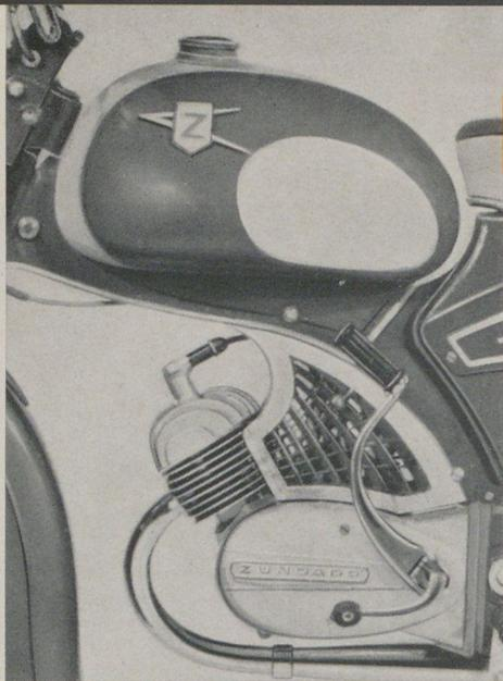
ZÜNDAPP 4-speed engine, two-stroke, 75 cc, 5.6 h.p. at 6,600 r.p.m., light-alloy cylinder, two-stroke petrol mixture 25:1, flywheel magneto ignition 6 V, 30+15 W, brake light, horn, steel-ball selector gearing, giving four speeds and neutral, kick starter, foot pedal gear change, 4-plate oilbath clutch.
